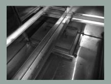
2. Place pump inlet screen in position-left rear corner of wash tank.
