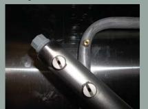
6. Wash and rinse nozzles must be inspected for blockage and cleaned.
