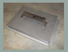
7. Pump inlet screen must be removed and cleaned thoroughly.
