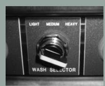
10. Turn wash selector to desired setting. (Light/5 min.
