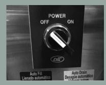
1. With Auto Drain: Push the auto drain button then wait 10 seconds and turn off the power switch. Without Auto Drain: Turn off power switch and open the drain valve.
